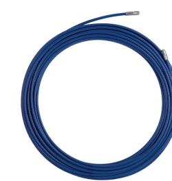
Steel spiral fish tapes are suitable for domestic cable installations, distances up to 20m and pipes up to  $\emptyset$ 23mm. Available in  $\emptyset$ 3,2mm without coating and in  $\emptyset$ 4mm and  $\emptyset$ 4,5mm with PVC
